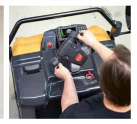
Ergonomically shaped controls, integrated into the innovative steering wheel, are easily reached by the operator without releasing his or her grip. The vibration-dampened steering unit is effortless to operate with either hand and is adjustable for optimized height and angle.
